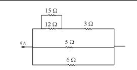
The voltage drop across the 5  $\Omega$  resistor in the portion of the circuit shown above is most nearly
