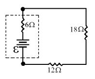
What is the total power dissipated by the external resistors in this circuit?
